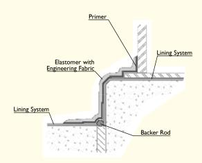
Seal for Tank Bottom and Foundation Treatment
