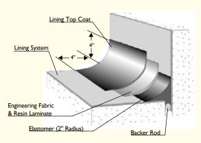
Joint Treatment Horizontal – Vertical Isolation Joint
